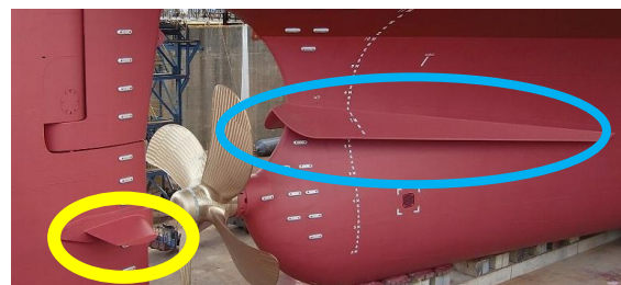
舵付きフィン(左黄色○)と Namura flow Control Fin(右水色○)
